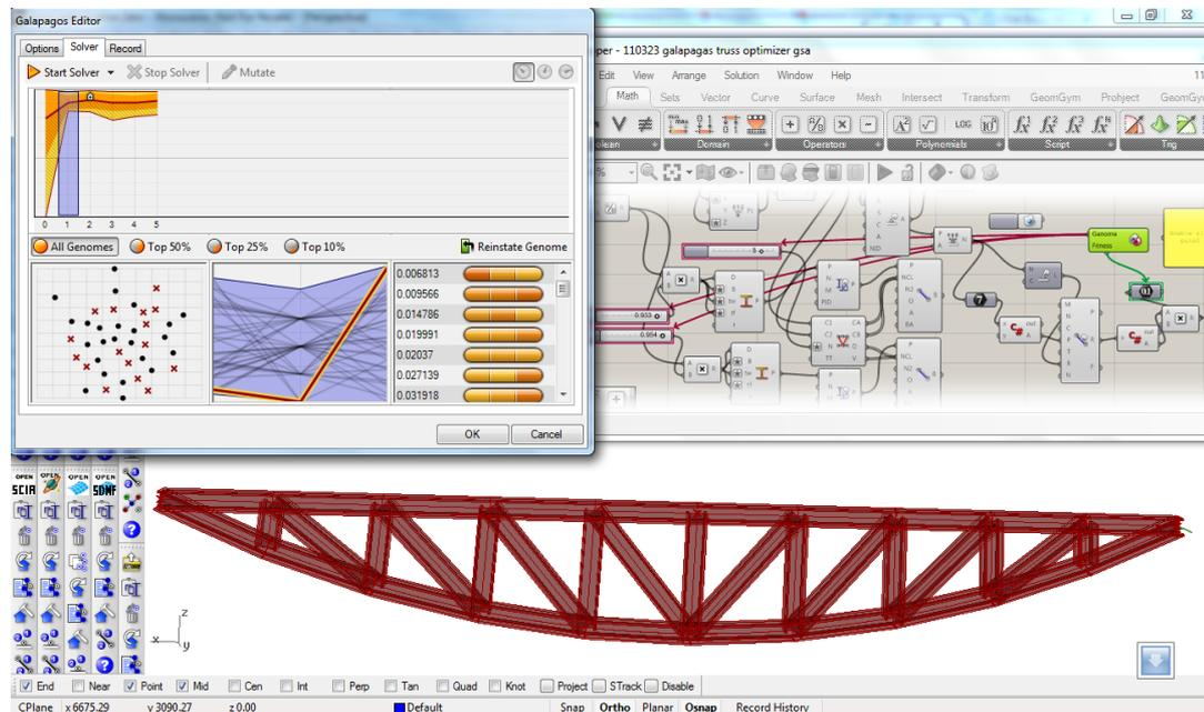
Fig. 13: Evolutionary Computing in progress using Galapagos, demonstrating Grasshopper problem/objective specification and solution progress for truss optimization.
