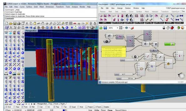
Fig. 1: IFC Model Manipulated generatively in Grasshopper3d
