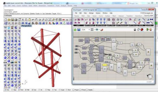
Fig. 10: Generative model form finding for tensegrity arrangement
